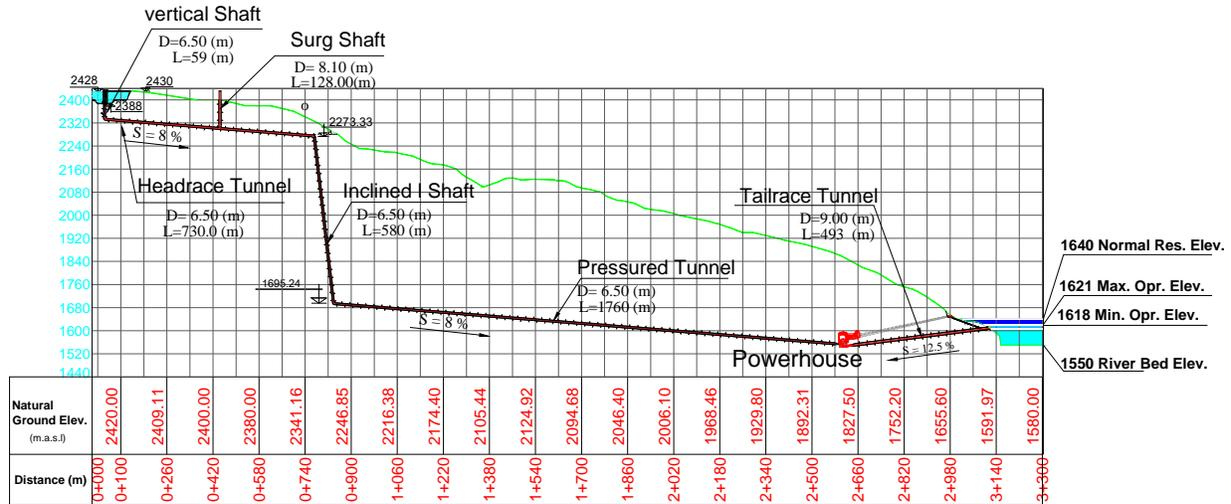
Fig 7. Longitudinal Section of Mirabad pumped Storage Hydro Power
